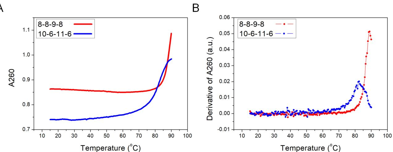
**Figure S9-2** Melting analysis of the RNA ssOrigami structures from Fig. 5E (10-6-11-6) and 5G (8-8-9-8). (A) The plot of raw data (A260 vs. temperature) of heating and cooling curves in red and blue, respectively. (B) The plot of the first derivative of A260 as a function of temperature.
