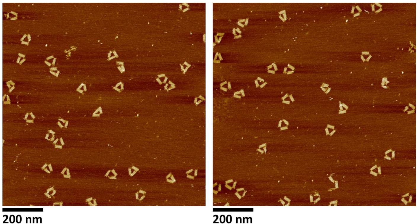
**Figure S11-6.** Additional AFM images for triangle-shape ssOrigami structures
