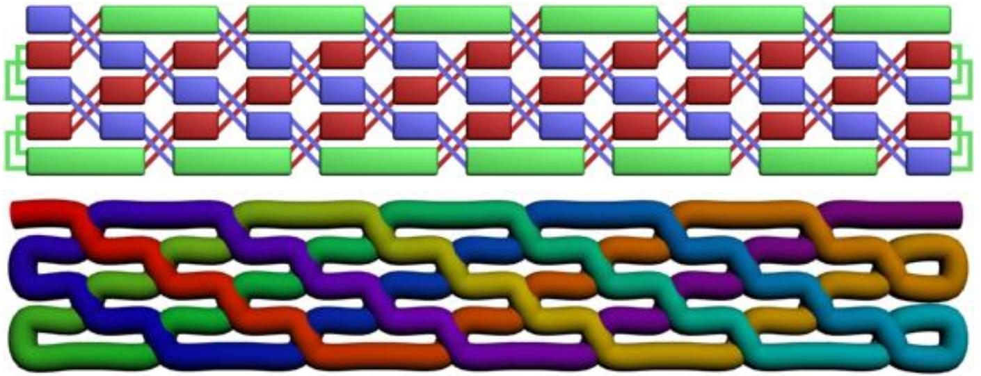
**Figure S5-5.** Cartoon (top) and pipeline style (bottom) model of the strip-shape ssOrigami design. The long green rectangles in the cartoon model stand for 26bps helical domains. The pipeline style model is colored with rainbow gradient starting from the 5' and 3' ends (red) to the middle of the strand (purple).
