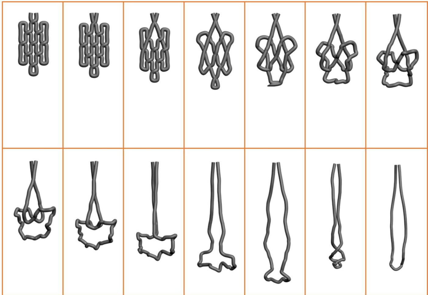
**Figure S5-8.** Selected screenshots of dynamic relaxation to demonstrate the knot relaxation process of our  $3 \times 3$  ssOrigami model. Relaxation movies are available in the supplementary information package [Movie-10].
