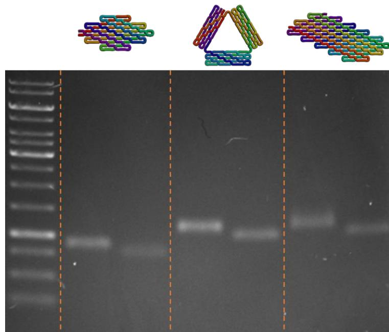
**Figure S7-3.** Native agarose gel characterization of cloned ssDNA product. For each sample, left lane contains ssDNA before annealing, and right lane contains ssOrigami after annealing.
