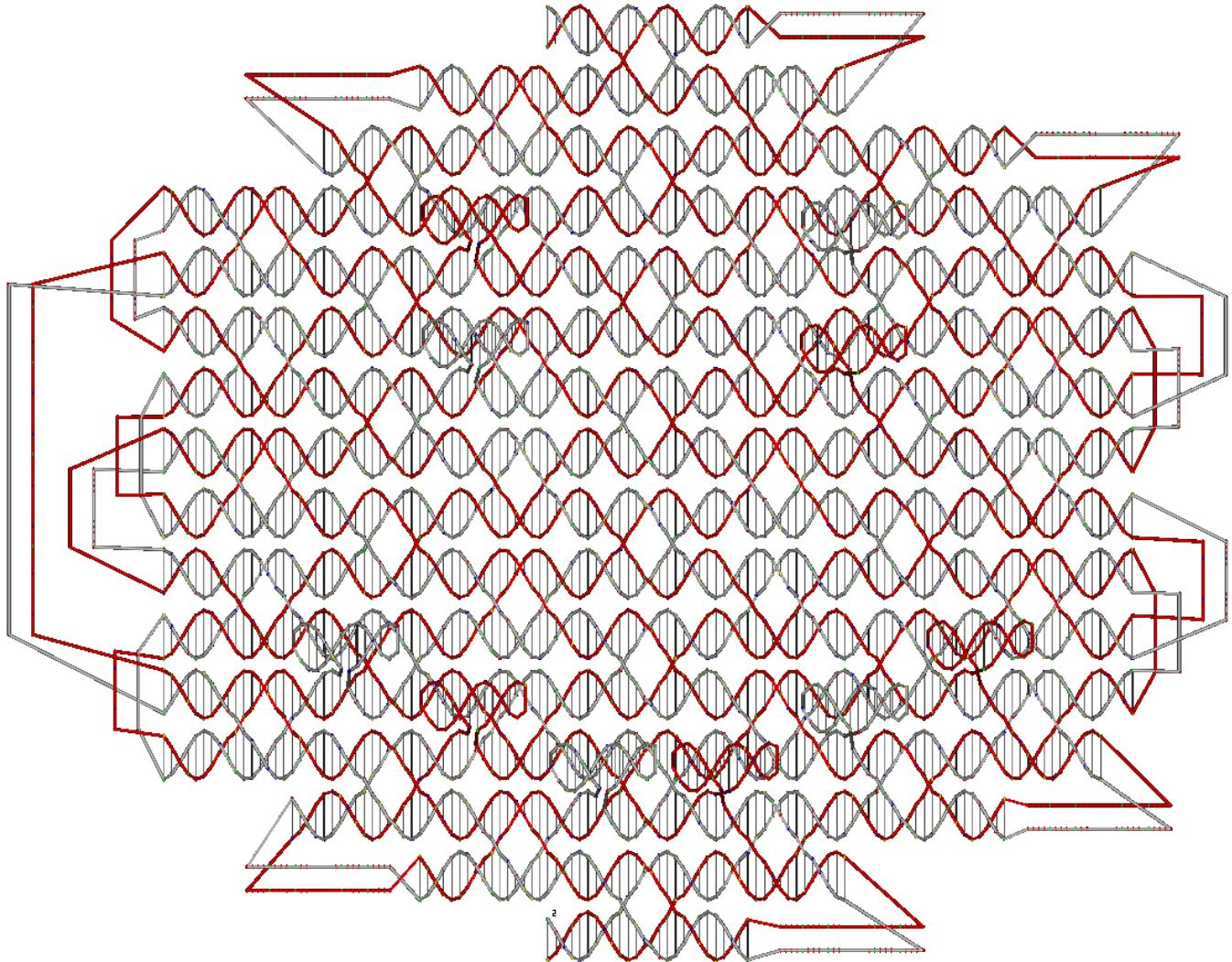
**Figure S12-10.** Design detail of hexagon shape ssOrigami with patterned smile face. Red strand is the forward strand and gray strand is the reverse strand.
