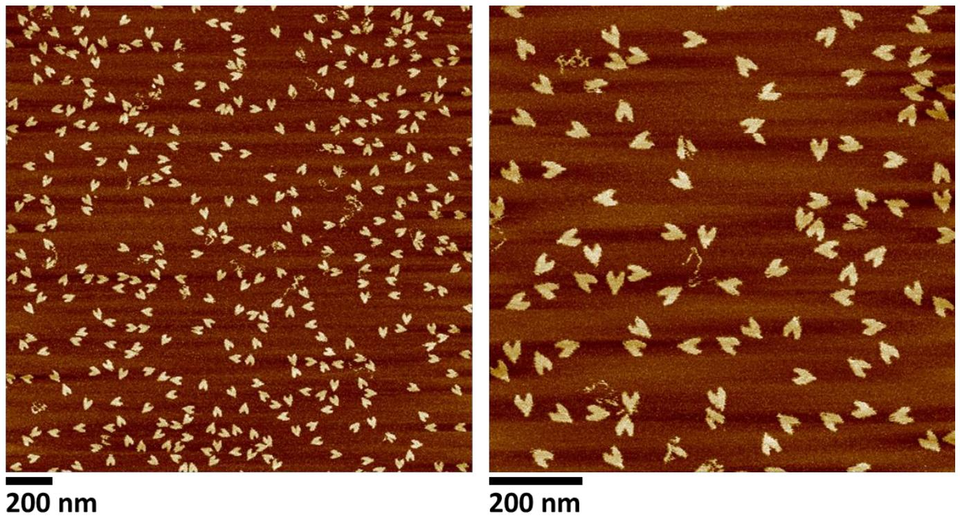
**Figure S11-5.** Additional AFM images for heart-shape ssOrigami structures
