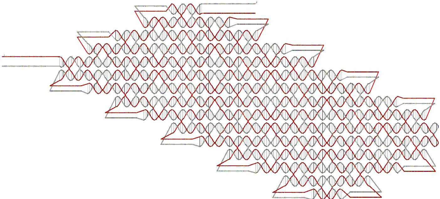
**Figure S12-4.** Design detail of  $5 \times 10$  rhomboid-shape ssOrigami. Red strand is the forward strand and gray strand is the reverse strand.
