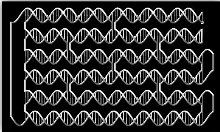
**Figure S3-1.** 2D projection of a typical anti-parallel ssOrigami design with ~800 nt.
