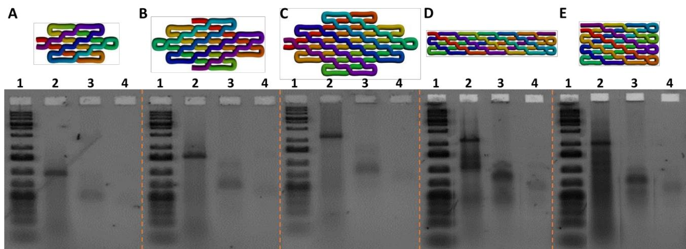
**Figure S6-2.** Agarose gel images of example ssOrigami products. Lane 1: 1 Kb ladder; lane 2: PCR product; lane 3: exonuclease treated product; lane 4: annealed products. In some cases, the concentration of folded DNA is too low to
