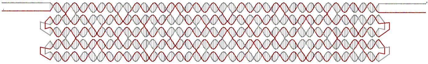
**Figure S12-7.** Design detail of strip-shape ssOrigami. Red strand is the forward strand and gray strand is the reverse strand.
