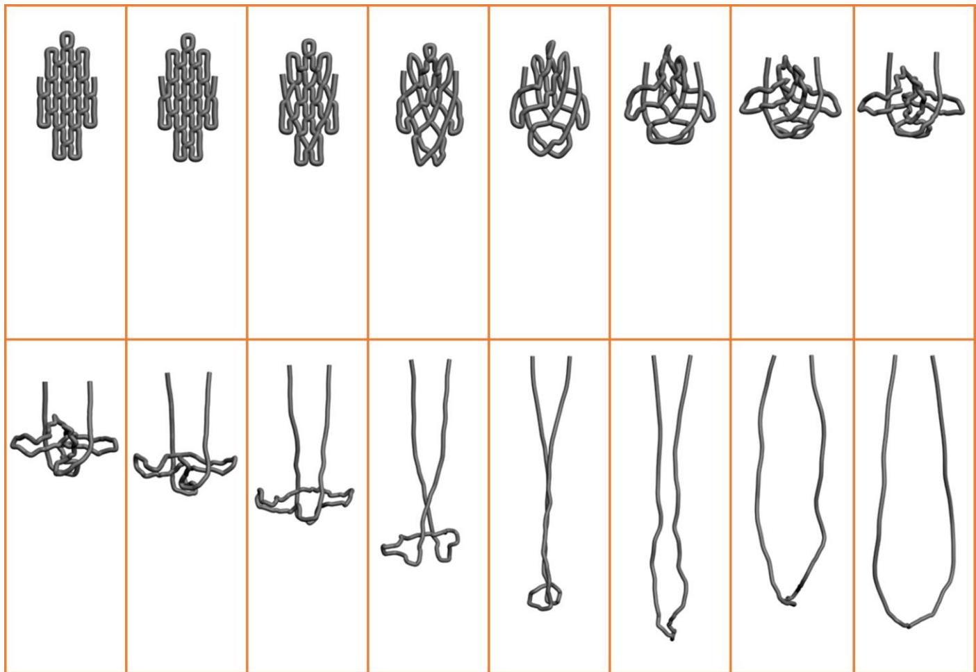
**Figure S5-9.** Selected screenshots of dynamic relaxation to demonstrate the knot relaxation process of our  $4 \times 4$  ssOrigami model. Relaxation movies are available in the supplementary information package [Movie-11].
