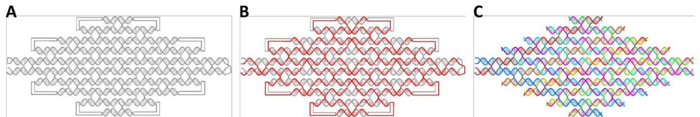
**Figure S10-1.** Models of  $5 \times 5$  diamond-shape designs constructed from single-strand (**A**), two half strands (**B**) and twenty short strands (**C**).
