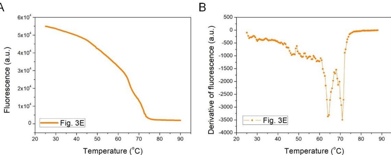
**Figure S9-1** Melting analysis of the heart-shaped ssDNA origami in Fig. 3E. (A) The plot of raw data (SyBr Green intensity vs. temperature) of the melting curve. (B) The plot of the first derivative of SyBr Green intensity as a function of temperature.
