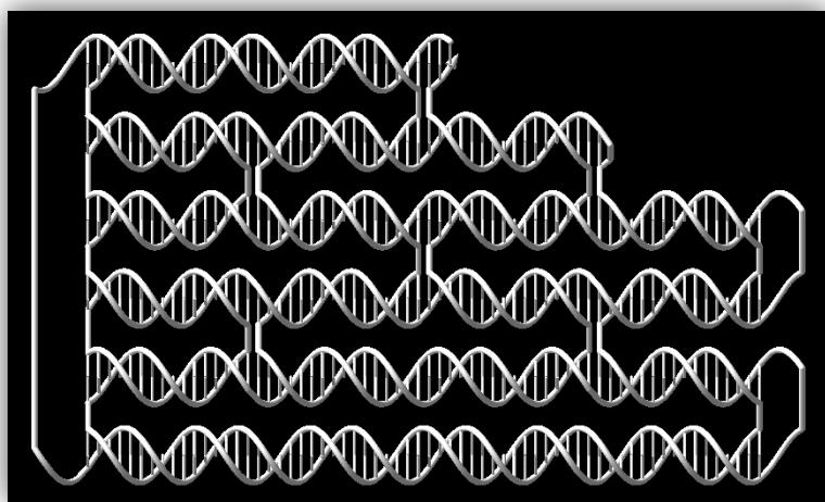
**Figure S3-4.** 2D projection of a typical anti-parallel ssOrigami design pattern.
