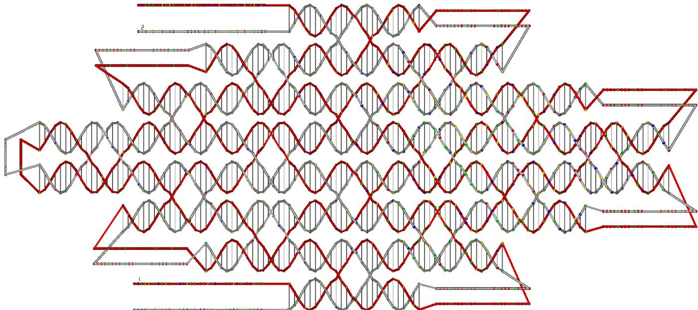
**Figure S12-2.** Design detail of  $4 \times 4$  diamond-shape ssOrigami. Red strand is the forward strand and gray strand is the reverse strand.
