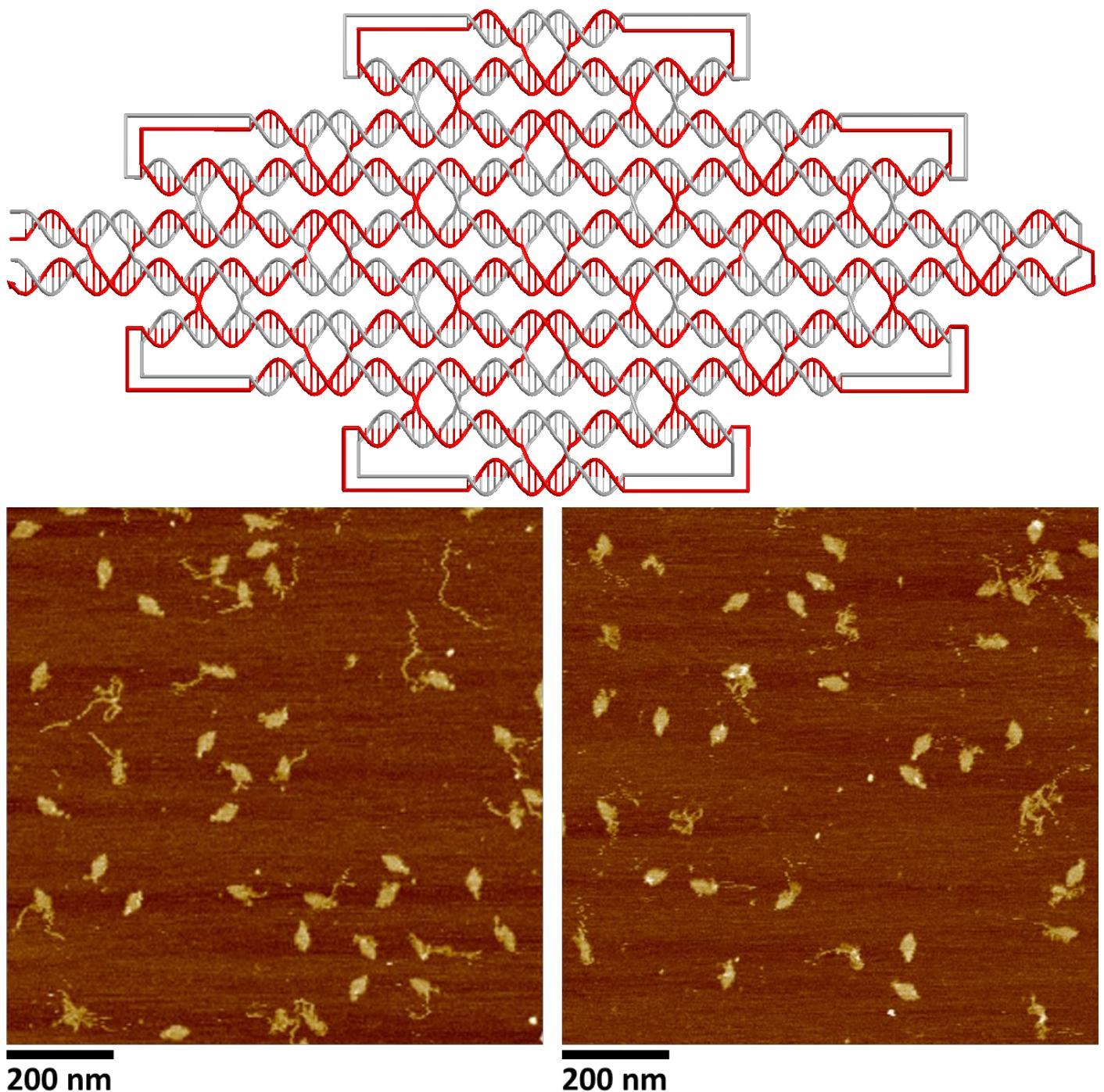
**Figure S10-2.** Model (top) and AFM images (bottom) for  $5 \times 5$  diamond-shape ssOrigami structures self-assembled from two half strands (not connected).
