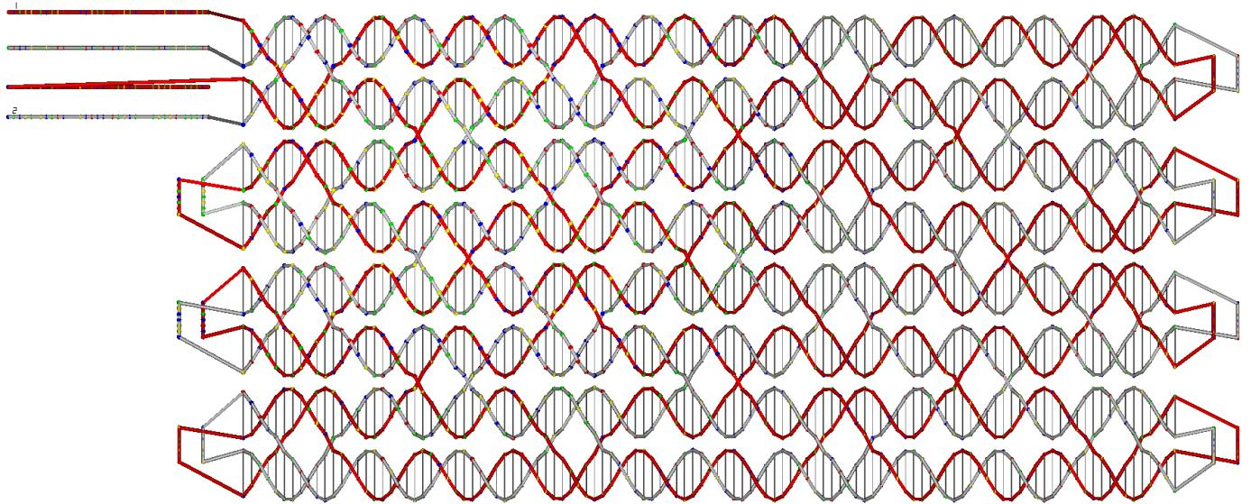
**Figure S12-12.** Design detail of rectangle RNA ssOrigami with 6bps locking domains. Red strand is the forward strand and gray strand is the reverse strand.
