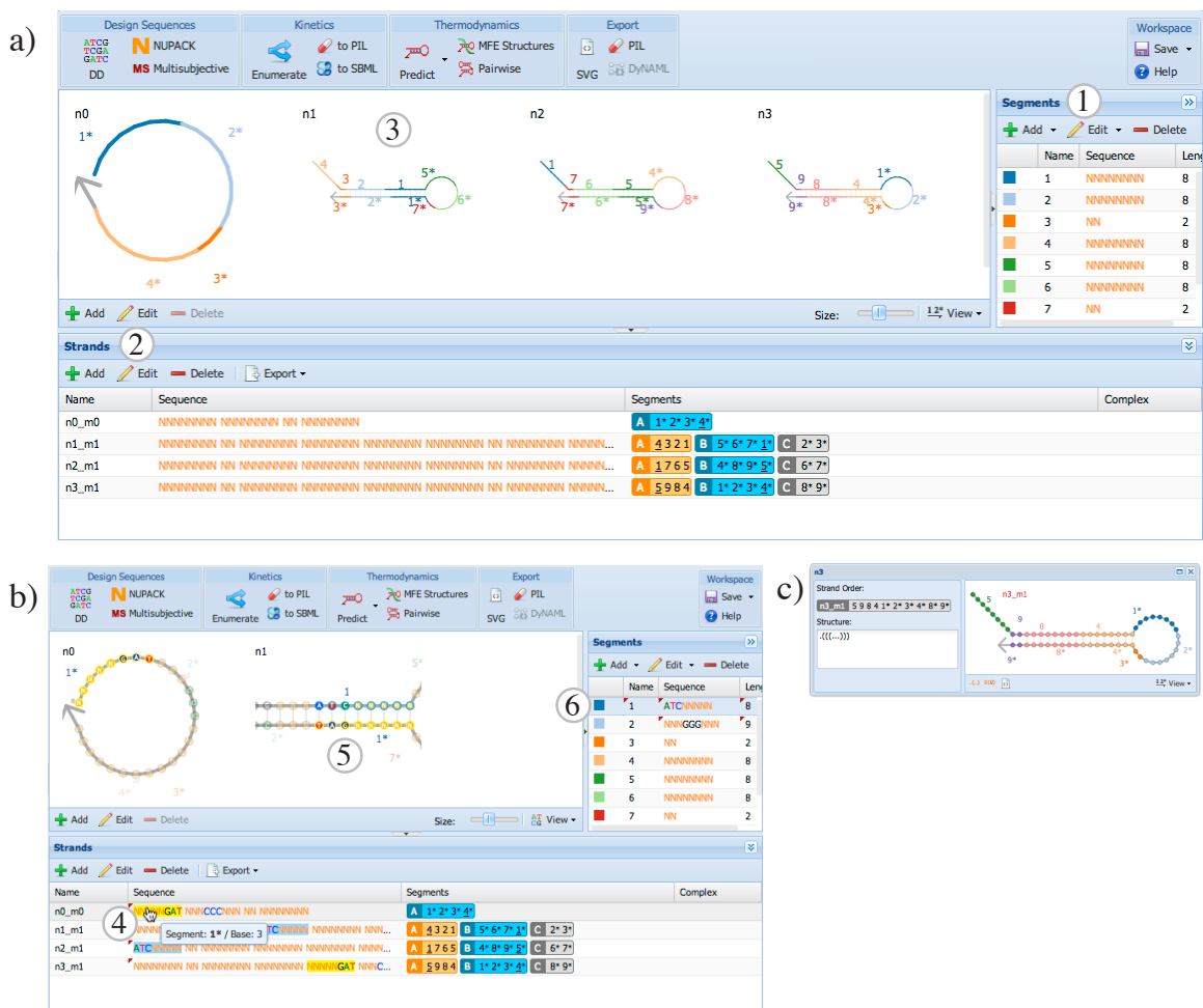
Figure S2: Segment-level (tier 2) design interface. (a) Users may view a preview of each of the segments ①, strands ②, and complexes ③ generated from the Nodal-level description. Segments, strands, and complexes may be edited in this view. Sequence constraints can be added to the design, or previously-designed sequences can be visualized on the structure. Individual bases in segments may be colored by segment identity, domain role (as in the Nodal view), or base identity (A, T, C, or G), and various view options may be specified. Segment-level designs may be exported to a variety of formats, or may be sent to sequence designers. Segment-level reaction enumeration, as well as sequence-level thermodynamic calculations, may be performed. (b) The user may point to segments ④ to highlight their appearance elsewhere in the design and interface ⑤, ⑥, making it easy to see where sequences (yellow) and their complements (light blue) propagate to other strands or species. (c) Complexes may be edited by selecting or re-arranging their constituent strands, or by modifying their secondary structure.
